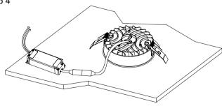
Make sure the downlight fixed tightly in ceiling, turn on the power.
