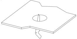
Open a hole according to the cutout size of led downlight.
