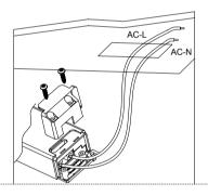
Use screw-driver to open the driver terminal cover, feed the main AC wire L. N. in terminal block respectively, then fix the cover back
