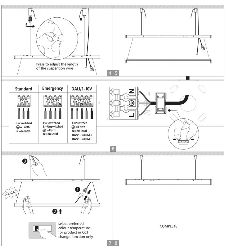
Wire diameter: 1.5 mm<sup>2</sup> splicing to 1350W max.
