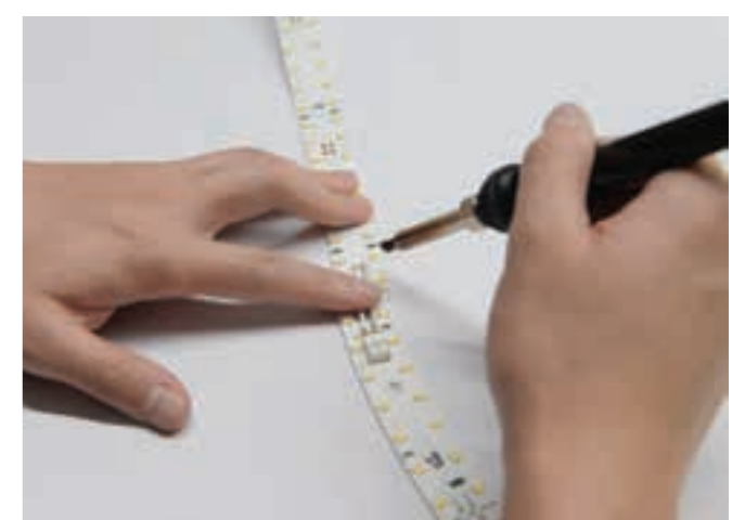
Insert the single-core cable into the WAGO connector and solder.
