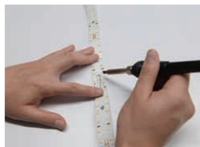
Align the LED strips and solder.(Pay attention to the positive and negative poles)
