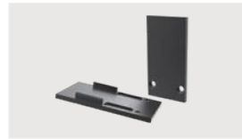
Model: GCTLEC-MH20 Material: ADC12 Size: L52×W27.2×H5.5mm Applicable model: GCTL-R20-MH2X0
