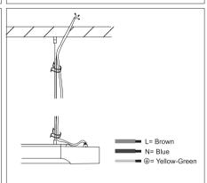
6. Connect to the power supply, installation complete.
