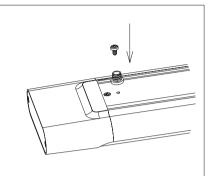
3. Fix the pedestal of installation ropes on the lamp using screws.
